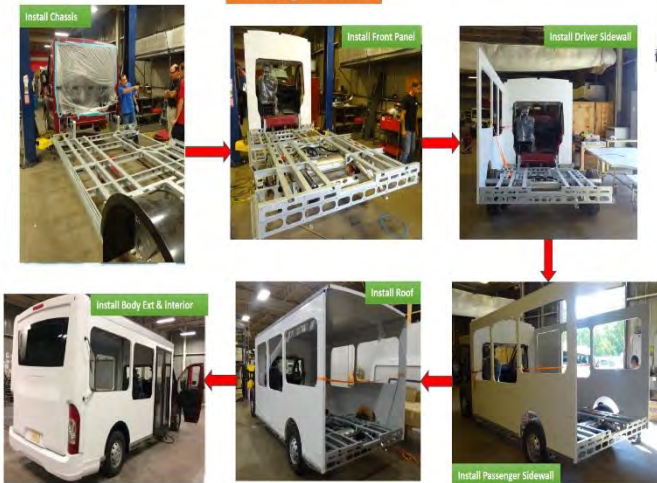
Bus Building Process Flow
